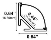
Width (outside): 0.64" (16.30mm) Width (inside): 0.44" (11.00mm) Height: 0.64" (16.30mm) Length: 0.96" (2.44mm)
