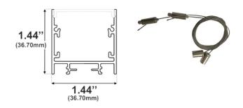
Width (outside): 1.44" (36.70mm) Width (inside): 1.18" (30.00mm) Height: 1.44" (36.70mm) Length: 0.96" (2.44mm)
