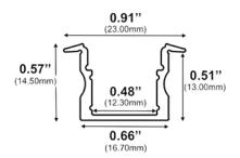
Width (outside): 0.91 (23.00mm) Width (inside): 0.48" (12.30mm) Height: 0.57" (14.50mm) Length: 0.96" (2.44mm)
