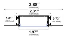
Width (outside): 1.97" (50.00mm) Width (inside): 1.77" (45.00mm) Height: 0.61" (15.50mm) Length: 0.96" (2.44mm)
