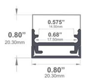
Width (outside): 0.80" (20.30mm) Width (inside): 0.68" (17.50mm) Height: 0.80" (20.30mm) Length: 0.96" (2.44mm)
