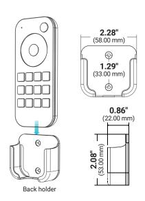
Back holder with magnet (The remote with built-in magnet)
